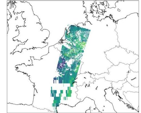
**CO2M:** constellation of satellite+instrument operated by ESA starting in 2026. Takes the best of TROPOMI (swath) for CO<sub>2</sub>. CO<sub>2</sub> column estimated in **clear skies, sunlit**.
