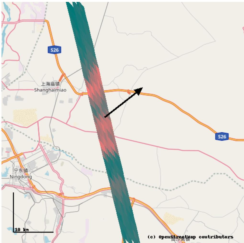
**OCO-2:** satellite+instrument operated by NASA since 2014, polar orbit, narrow swath. **Ground resolution = 3 km<sup>2</sup>.** **Column-average CO<sub>2</sub> concentration estimated in clear skies, sunlit.**
