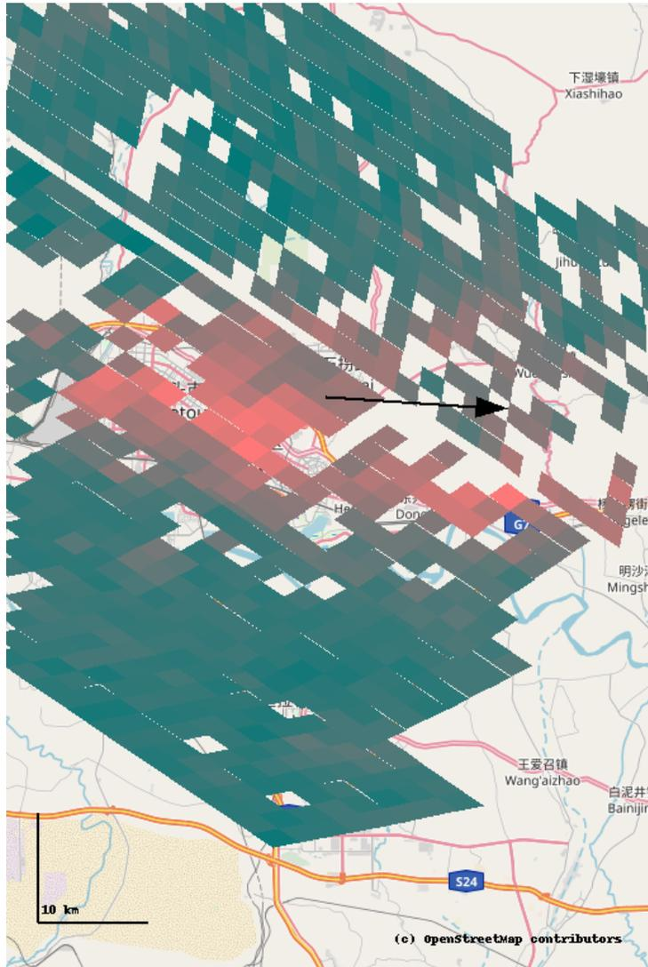
**OCO-3:** instrument operated by NASA onboard the International Space Station since 2019, narrow swath but a same scene can be scanned successively several times. **Ground resolution = 3 km<sup>2</sup>. Column-average CO<sub>2</sub> concentration estimated in clear skies, sunlit.**
